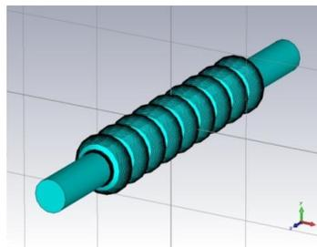
Figure 1: Geometry of the third harmonic 3.9 GHz cavity.
