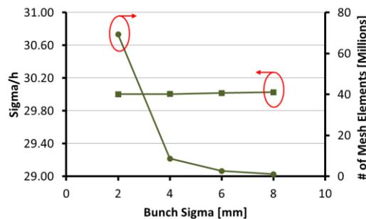
Figure 2: Sigma/h and number of mesh elements vs. bunch sigma.
