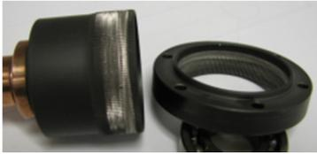
Figure 8: Harmonic drive gear failure.
