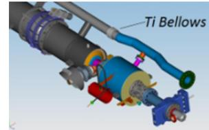
Figure 10: Ti bellows between magnet and cavity #8.
