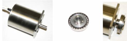
Figure 6: Harmonic drive wave generator connection to the motor shaft.
