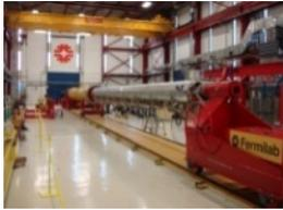
Figure 3: CM2 cold mass on the Big Bertha fixture.
