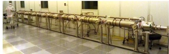
Figure 1: CM2 cavity string in the cleanroom.
