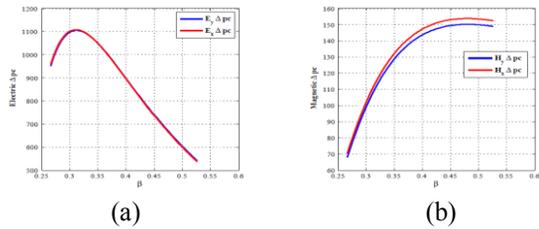
Figure 8: SSR2 Y-spoke transverse kicks vs. beta, (a) electric and (b) magnetic.
