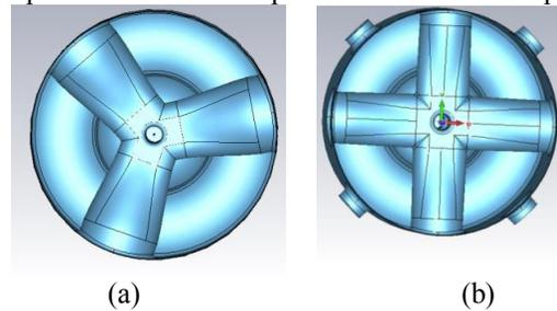
Figure 5: (a) Y-spoke design cross section, (b) X-spoke x-y section.
