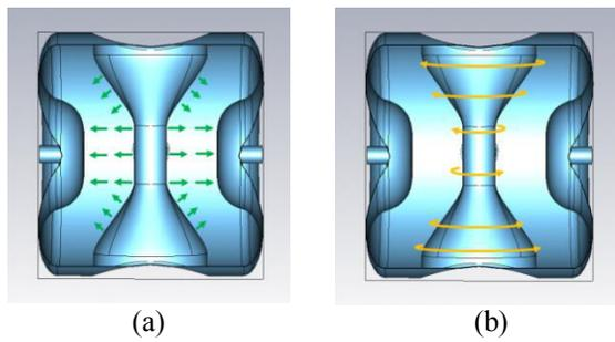
Figure 2: field line sketch of a spoke resonator (a) electric and (b) magnetic [1].
