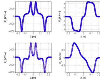
Figure 1: SSR2 electric and magnetic transverse fields.
