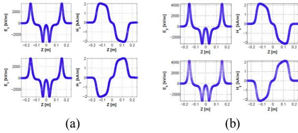
Figure 6: SSR2 transverse field on 10 mm offset (a) Y-spoke, (b) X-spoke.
