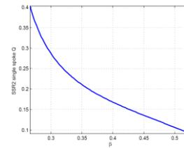
Figure 4: SSR2 single spoke asymmetry parameter vs. particle beta
