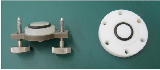
Figure 3: Left, new BCP blank flange design. Right, old BCP blank flange design.
