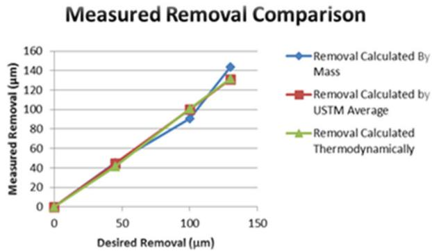
Figure 5: Comparison of measurement techniques for each stage of  $\beta=0.53$  cavity bulk etch.
