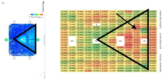
Figure 4: Left, Predicted flow pattern. Right, resulting etch removal measured by USTM.
