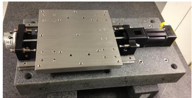
Figure 10: 112 MHz FPC linear motion system.
