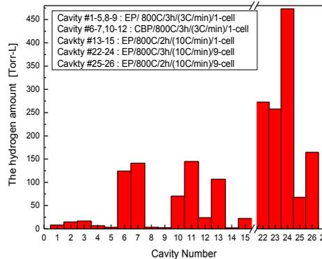
Figure 4: Comparing degassed H<sub>2</sub> in single-cell vs. nine-cell cavities.
