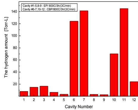
Figure 3: Comparing degassed H<sub>2</sub> in electropolished vs. tumbled cavities.
