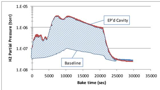
Figure 2: Area between the cavity and baseline H<sub>2</sub> pressure curves.
