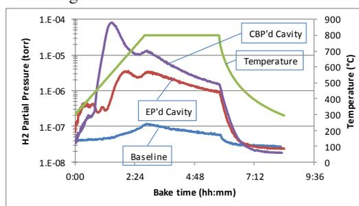
Figure 1: Typical H<sub>2</sub> partial pressures of an electropolished cavity, a tumbled cavity, and an empty chamber within 300°C to 300°C.
