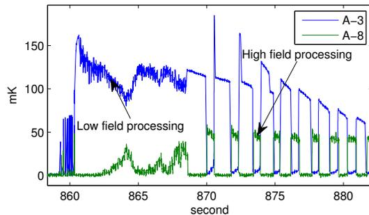
Figure 5: MP processing happened at A-3 and A-8 sensor when peak magnetic field approached 95 mT. The sudden "turn on" of the processing is shown with pulse heating changing into a continuous heating signal.
