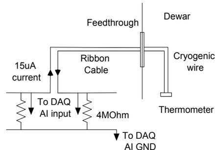
Figure 3: Schematic of the measurement circuit. A  $15\ \mu\text{A}$  current is used to excite the thermometer, and the voltage drop across the resistor is used to measure the resistance value.
