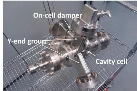
Figure 1: The APS superconducting deflecting cavity during assembling in a clean room. The cavity has a Y-end group on the beam pipe and a on-cell waveguide damper.
