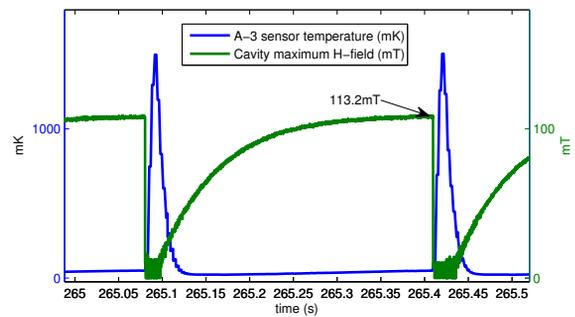
Figure 6: Quench pulse heating signal, the quench location temperature heating can go as high as 1.5K.
