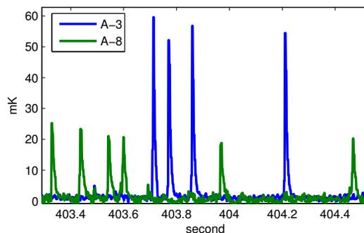
Figure 4: A soft MP barrier occurred at the A-3 and A-8 sensors when the maximum surface M-field approached 85 mT. Pulse heating can be detected when MP occurs
