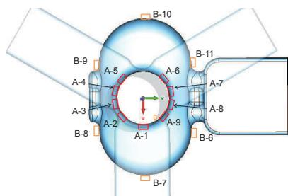
Figure 2: Sensor layout around the cell and the iris looking from the Y-end group side. The iris on the other side has similar sensors around the iris.
