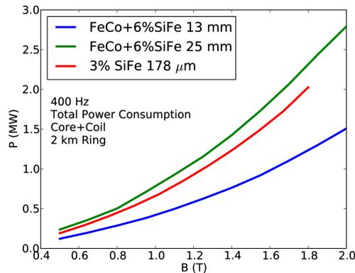
Figure 6: Total power loss for entire ring.
