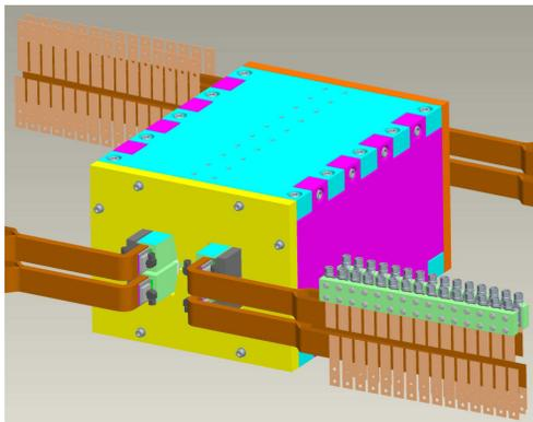
Figure 7: Rapid cycling dipole assembly.
