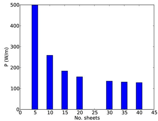
Figure 4: Power loss per m of magnet for different numbers of conducting sheets.
