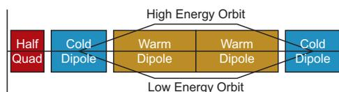
Figure 1: Structure of a quarter cell, showing the expected deviation of high and low energy closed orbits.
