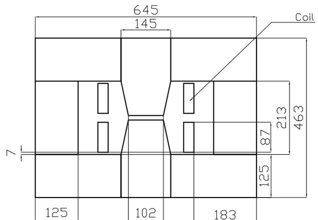
Figure 2: Geometry of the dipole magnet (in mm).
