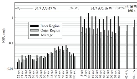
Figure 1: Typical NZP velocities measured in test 2G wire coils [4].
