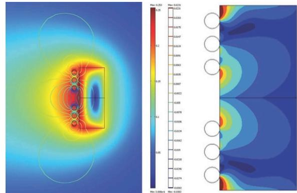
Figure 3: AC magnetic fields (left and shaded), DC magnetic fields (right contours) of the fabrication optimized simulations.
