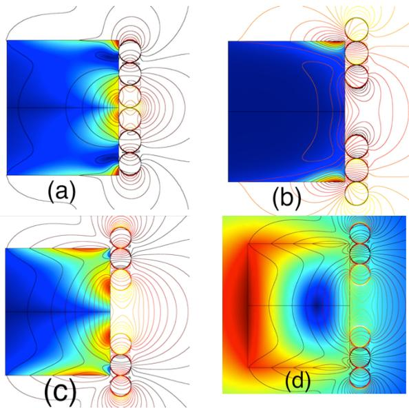
Figure 2: Resonant coil optimization showing field penetration color map and AC field contour map with initial geometry configuration (a), 1000Hz operation (b), final optimized geometry and frequency (c) and final DC magnetic field color map and AC field contour map (d).
