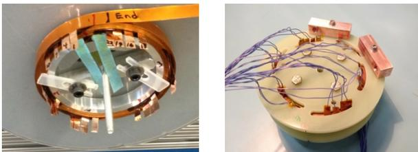
Figure 4: HTS coil on the winding fixture and shown with soldered voltage taps (left). Double pancake coil stack shown with tap leads soldered on and copper warm lead blocks.
