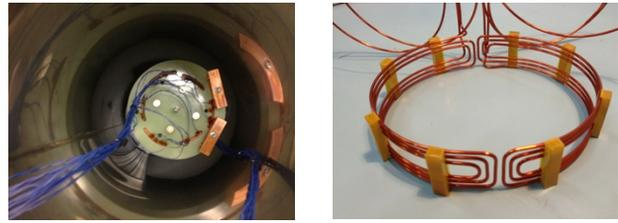
Figure 5: HTS coil placed cryochamber (left), resonant coils prior to forming around HTS coils (right).
