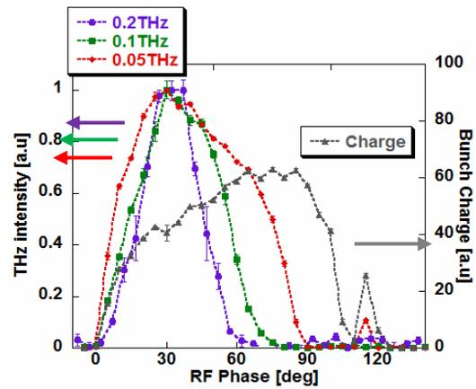
Figure 11: Phase dependence of several detectors.
