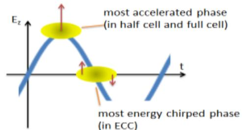
Figure 2: Off-crest acceleration in ECC.
