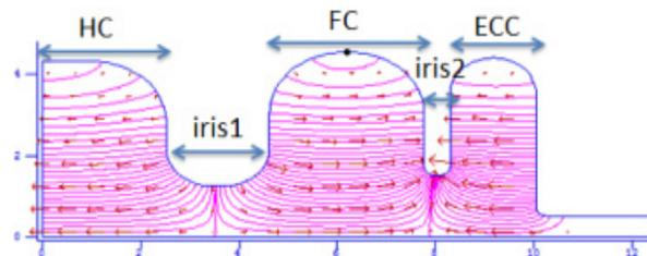
Figure 1: The cavity structure of the ECC RF gun.
