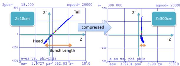
Figure 3: The longitudinal phase space distribution right after ECC (left), distance of 3m from cathode (right).
