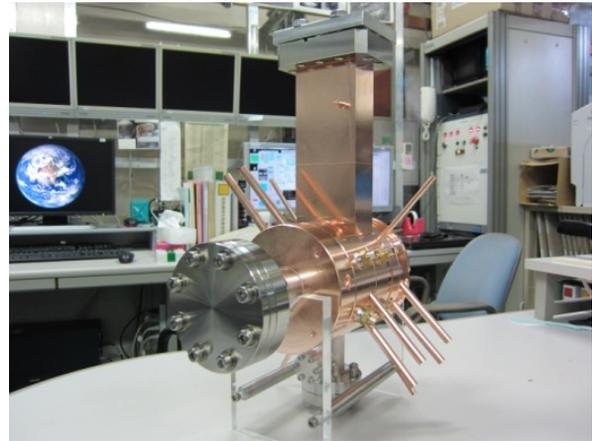
Figure 6: Manufactured ECC RF gun.
