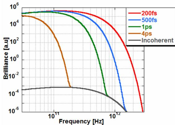
Figure 9: CSR spectrum calculated by SPECTRA (3.7MeV, 100pC).
