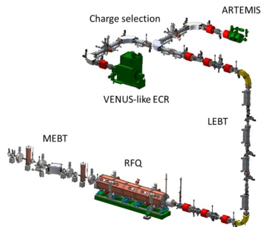
Figure 1: FRIB Front End layout.
