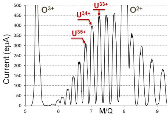
Figure 2: VENUS M/Q intensity scan for a uranium beam, demonstrating world record intensity of charge states 33+ and 34+.
