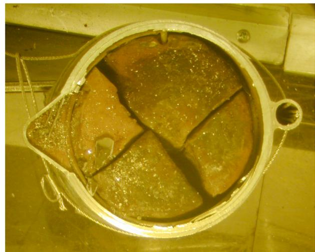
Figure 1: Broken and corroded Lujan Center tungsten target (from [1]).
