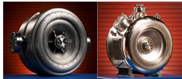
Figure 9: SSR1 cavity, bare (left) and dressed (right).
