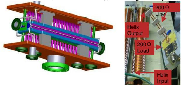
Figure 5: The MEBT kicker. A 3D model of the 50-Ohm kicker (left). Part of the vacuum box is removed for the presentation purpose. A model of the 200 Ohm kicker (right).
