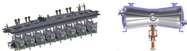
Figure 7: HWR CM design: a cavity-solenoid string attached to the top lid (left), a cavity with a coupler (right).
