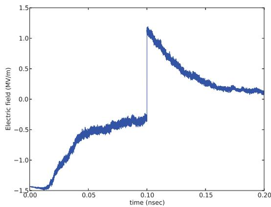
Figure 2: Electric field at diamond surface versus time.
