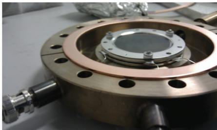
Figure 7: Multi Channel Plate Detector
