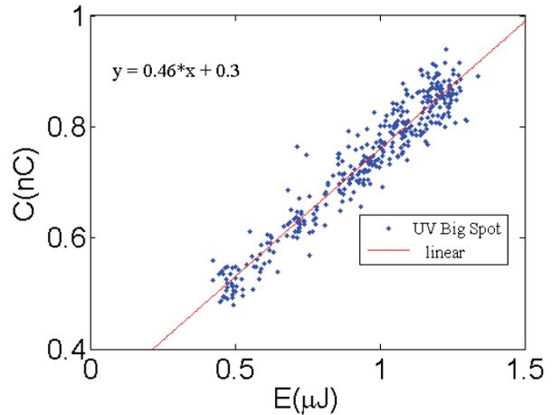
Figure 6: Charge vs. UV laser energy for  $Cs_2Te$  (single photon emission).
