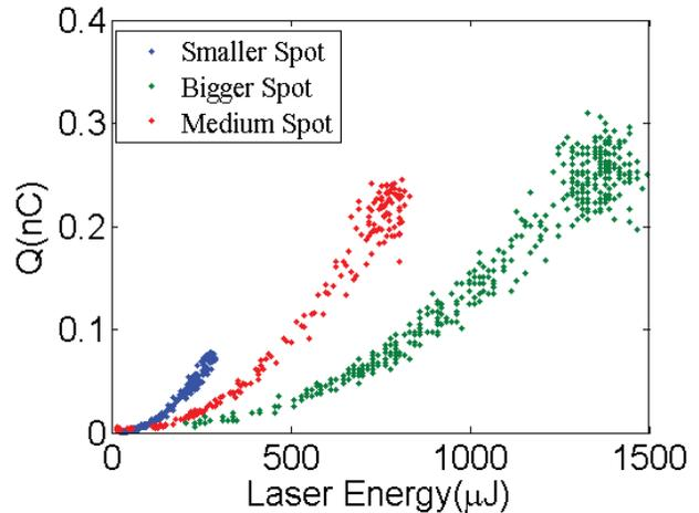
Figure 3: Charge variation as a function of laser energy for the three laser spot sizes considered in Fig. 2.
