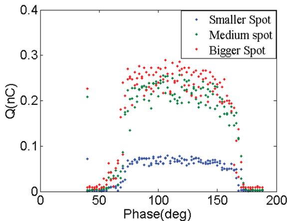
Figure 2: Charge dependence on laser phase relative to the gun (with an arbitrary phase offset). The blue, green, and
