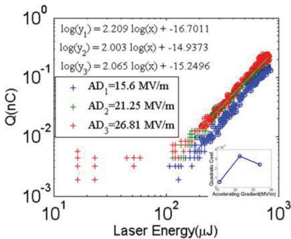
Figure 5: The effect of the accelerating gradient on the charge yield. Inset: The variation of the quadratic coefficient with the accelerating gradient.
