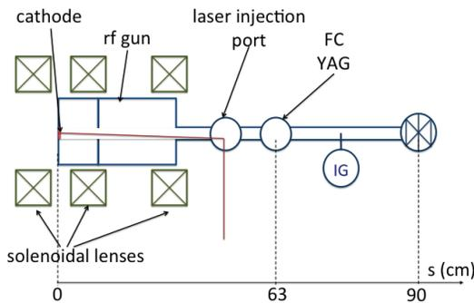
Figure 1: Overview of the HBESL electron source area. The IR pulse is injected through the laser injection port. The legend is FC: Faraday cup, IG: ion gauge, YAG: Yttrium Aluminum Garnet scintillating screen.
