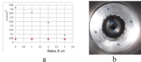
Figure 5: a) Ion emission current density  $J_i$  (A/cm<sup>2</sup>) (plasma density) along the radius  $R$  (cm) at high magnetic field (blue) and at low magnetic field (brown) with RF power 1.5 kW in the plasma (observed by small collectors) without transverse magnetic field  $B_t$ . b) Trace of plasma flux on the collar converter wall with transverse magnetic field  $B_t \sim 1$  kG concentrated up to 8 mm of diameter.
