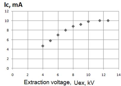
Figure 10: Dependence of the collector current  $I_c$  on the extraction voltage  $U_{ex}$ . RF power in the plasma  $P_{rf}=1.5$  kW, the solenoid voltage  $U_m=8.3$  V. Gas flow  $Q=8.6$  sccm.
