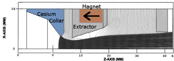
Figure 3: A schematic of ion beam formation (emission aperture is 6 mm diameter).
