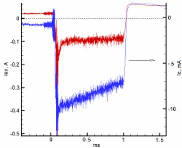
Figure 7: Signals from extractor  $I_{ex}=0.1$  A (electron current, red) left scale and signal from collector  $I_c=10$  mA (negative ion current, blue) right scale. Signal slope connected with a low inductance of the Pearson transformer.
