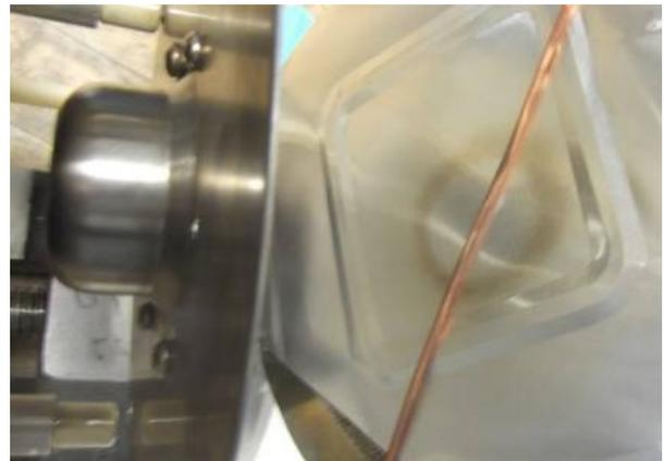
Figure 11: Accelerating electrode and a collector with a trace of sputtering by negative ion beams.
