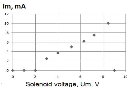
Figure 9: Dependence of  $I_c$  on the solenoid voltage  $U_m$ .
