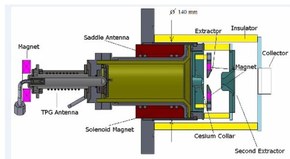
Figure 1: A schematic of the SA SPS with an extraction system and a collector.
