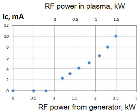
Figure 8: Dependence of  $I_c$  on RF power in the plasma  $P_{rf}$  (upper scale) and from generator (bottom scale).
