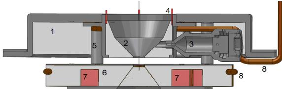
Figure 2: Extraction system of the RF SA SPS. 1- plasma electrode; 2-emitter/converter cone; 3-Cesium oven; 4- Cs cartridges; 5-ceramic insulators; 6- extraction electrode; 7- permanent magnet; 8-cooling tubes.
