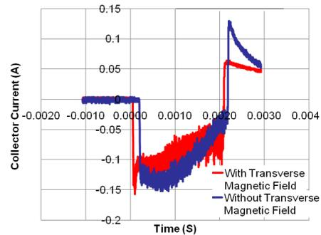
Figure 6: Traces of positive ion current to the collector with and without transverse magnetic field.
