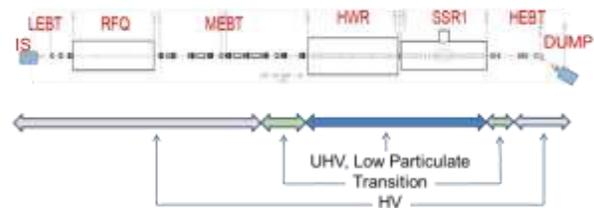
Figure 1: PXIE System Layout with classification of vacuum levels. HWR and SSR1 indicate location of two cryomodules.
