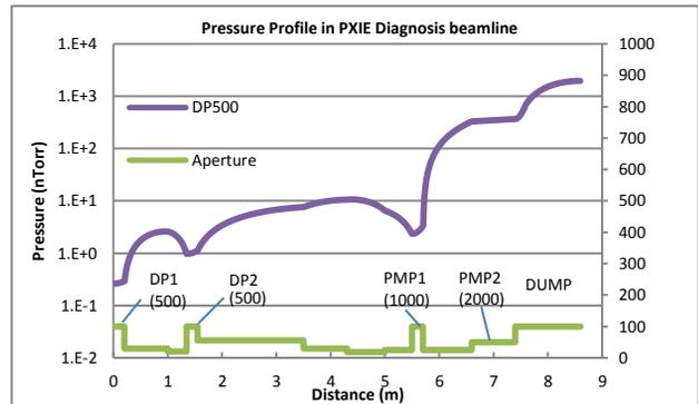
Figure 4: The pressure profile in HEBT-DUMP. The number in parentheses is pumping speed in l/s. there is no gas flow at the ends.
