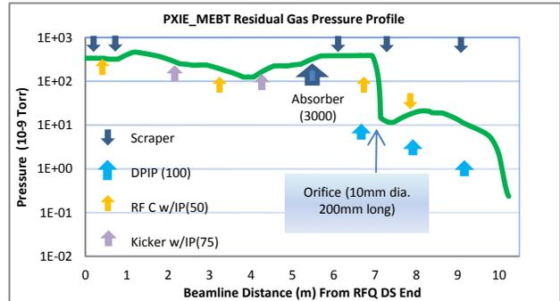
Figure 3: The pressure profile in MEBT. There is no gas flow at the both ends. The number in parentheses is pumping speed in l/s.
