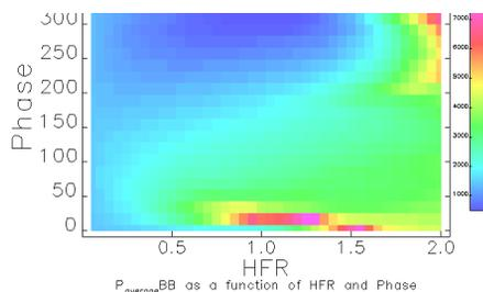
Figure 6: Back-bombardment simulation power as a function of harmonic field and the relative RF phase. The minimum is at 310 degrees and 1.1 HFR
