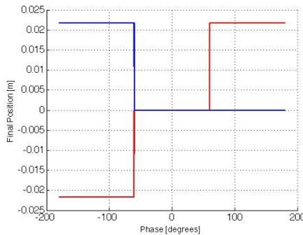
Figure 2: Ideal waveform (red) for complete back-bombardment mitigation with an overlay of its emission phase profile (blue).
