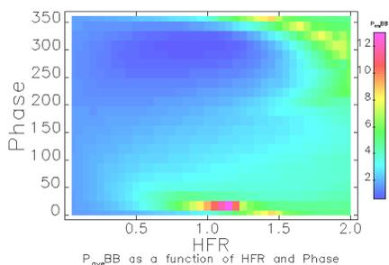
Figure 7: Back-bombardment as a function of the harmonic field ratio and the relative RF phase.
