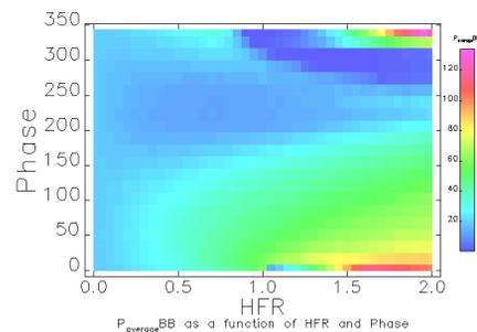
Figure 5: Theoretical result for the back-bombardment power as a function of the harmonic field ratio and the relative phase of the two RF powers.
