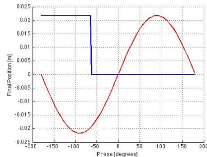
Figure 1: The resultant back-bombardment phase profile for a gap of 2cm and a RF frequency of 1.3GHz. Using a simple Newtonian model.
