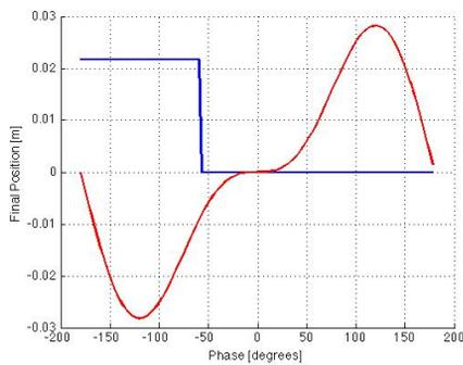
Figure 3: Phase profile for the two-frequency case using a simple Newtonian model (blue) with the temporal field envelope overlay (red).
