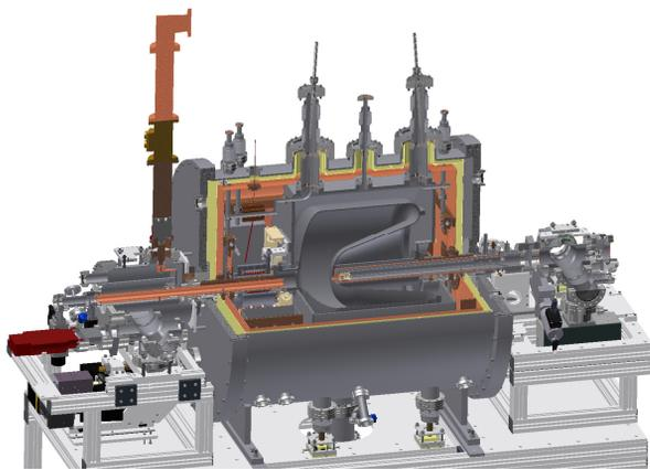
Figure 1: The photocathode, SRF cavity and high-temperature superconducting solenoid in the liquid-helium cryostat. Courtesy of G. C. Rogers.
