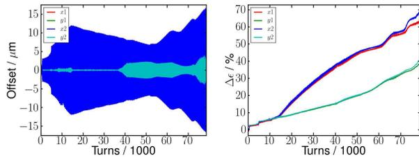
Figure 1: Case A, offset (left) and emittance growth (right) versus time.
