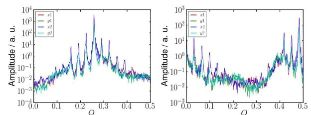
Figure 5: Case B, offset and envelope spectrum after 3000 turns.
