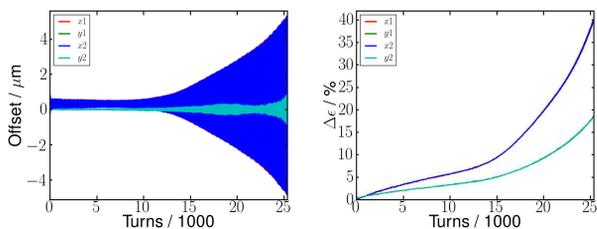
Figure 6: Case C, offset (left) and emittance growth (right) versus time.
