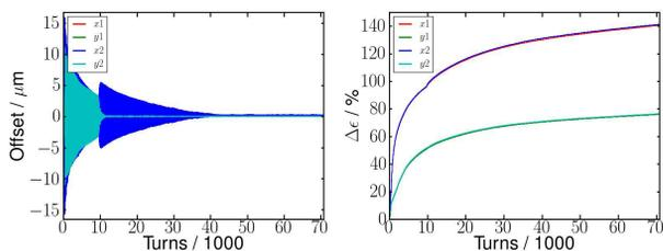
Figure 8: Case D, offset (left) and emittance growth (right) versus time.
