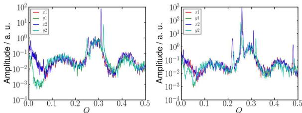
Figure 7: Case C, offset spectrum after 1000 turns and 20,000 turns. The  $\pi$  and  $\sigma$  beam-beam modes are clearly visible.
