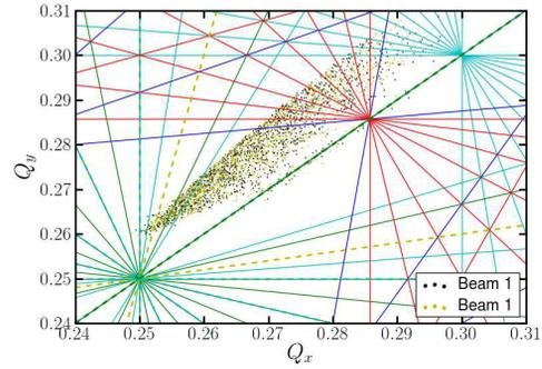
Figure 3: Case A, tune footprint. The visible resonance lines include 4<sup>th</sup> order (cyan dashed), 6<sup>th</sup> order (yellow dashed), 7<sup>th</sup> order (red), 8<sup>th</sup> order (green), 9<sup>th</sup> order (blue) and 10<sup>th</sup> order (cyan solid).
