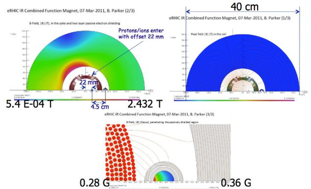
Figure 5: Combined function magnet with three different functions at the same time: bend the ions for 4.5 mrad, field free region for electron passage, and neutron detection downstream.
