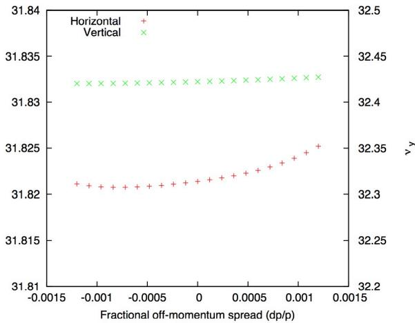
Figure 9: Tune dependence on momentum after sextupole correction
