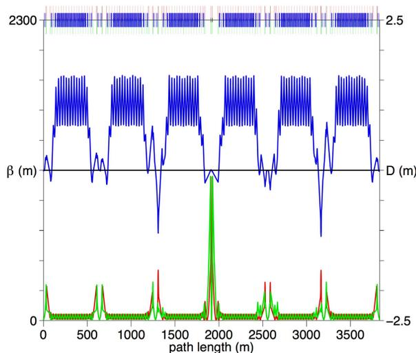
Figure 1: eRHIC lattice design with the  $\beta^* = 10$  cm at the single interaction region at 6 o'clock IP.
