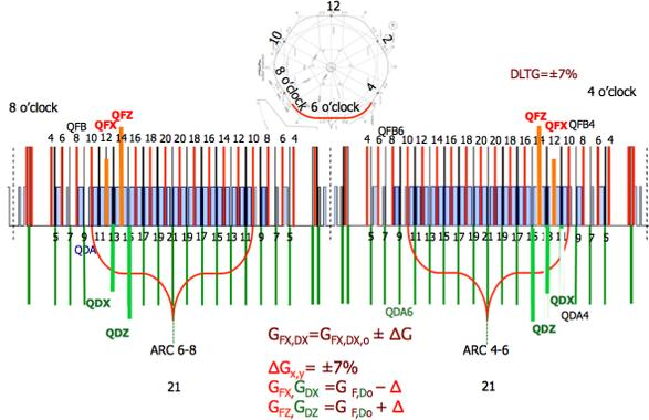
Figure 8. Sextupoles and pairs of quadrupoles used to create the wave in two arcs neighboring the IP.
