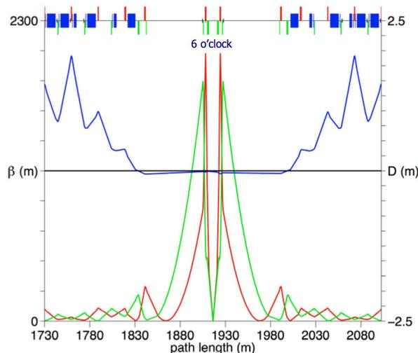
Figure 2: Details of betatron functions in the IR.
