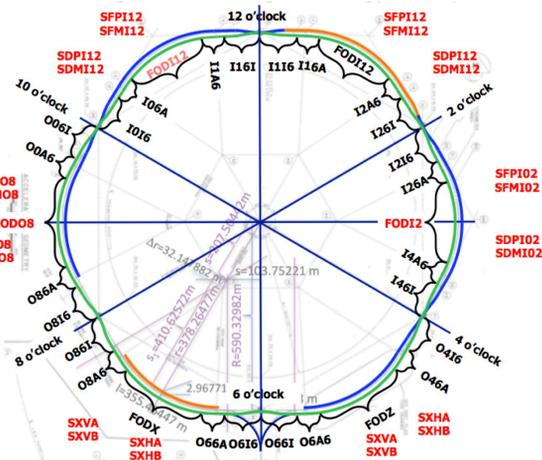
Figure 6: 24 families of sextupoles in the 90° degrees lattice are able to correct the first and higher orders of chromaticities in eRHIC lattice.
