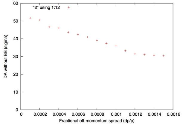
Figure 11: The dynamical aperture in the eRHIC lattice with  $\beta^* = 10$  cm after 24 family of sextupole correction.
