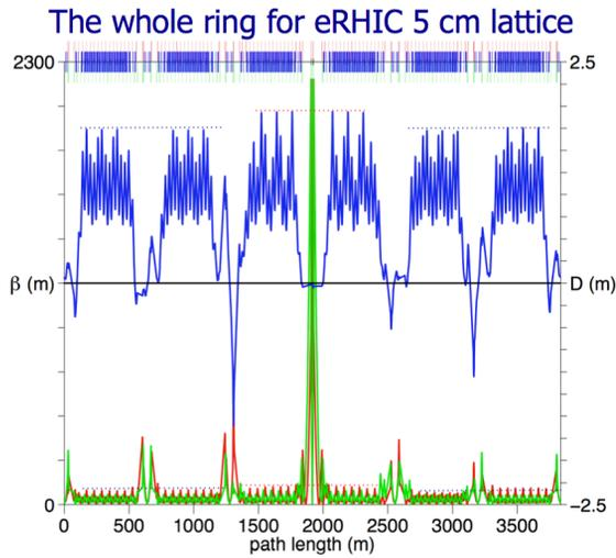
Figure 7. Betatron squeeze to  $\beta^* = 5$  cm.
