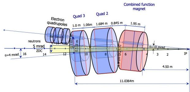
Figure 4: The triplets for both electron and ion lattice eRHIC IR layout with neutron solid angle (yellow).
