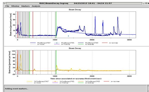
Figure 4: Comparison of beam loss between the test ramp and a physics ramp for both rings.
