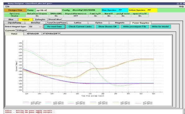
Figure 8: Current curves for selected magnets with ramp optics correction.
