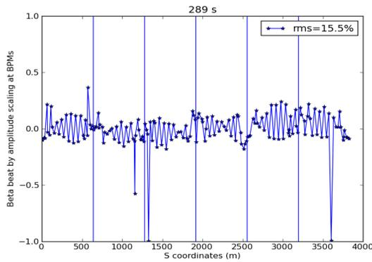
Figure 2: Beta beats at 289 s into ramp in the horizontal plane from ramp optics measurement.
