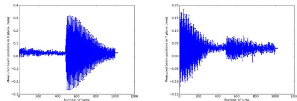
Figure 1: Turn by turn BPM positions in the horizontal (left) and the vertical (right) plane from ramp optics measurement, residual coupling (right) appears in the vertical plane where the horizontal oscillation starts.
