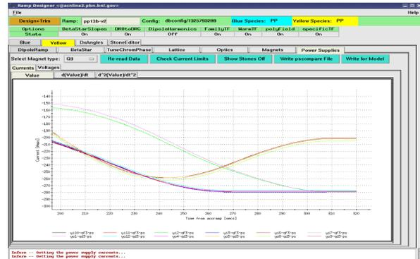
Figure 7: Current curves for selected magnets without ramp optics correction.
