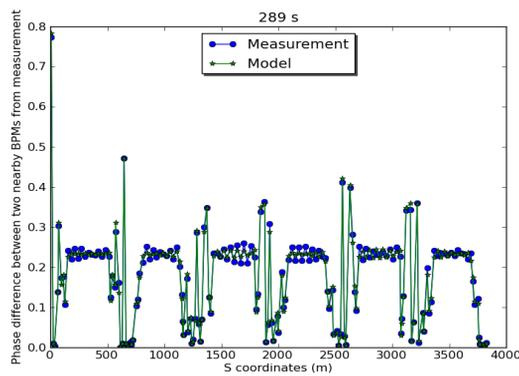
Figure 3: Phase errors at 289 s into ramp in the horizontal plane from ramp optics measurement.
