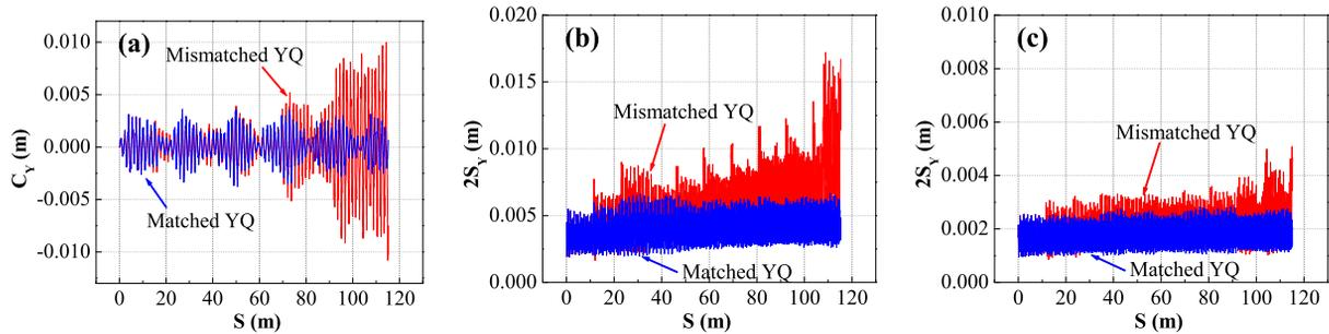
Figure 2: Results of calculations (*with* incoherent transverse space charge) in ELEGANT over 10 turns at (1.99, 1.99)A operating point in UMER: a) Vertical component of centroid motion for either 0.6 or 6.0 mA beams; b) 6.0 mA beam's vertical  $2\times$ rms semi-axis; and c) 0.6 mA beam's vertical  $2\times$ rms semi-axis. The strength of injection quadrupole YQ is increased by  $\sim 15\%$  to yield near-matched envelope conditions past  $\nu_{0y} = 7.5$ . The vacuum pipe radius is 0.025 m.
