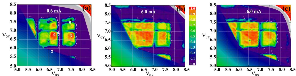
Figure 1: Beam lifetime charts at 10th turn as a function of estimated bare tunes ( $x$ : horizontal,  $y$ : vertical): (a) 0.6 mA beam (emittance dominated) with varying strength of injection quadrupole QR1 (see text and Table 1); (b) 6.0 mA beam (space charge dominated) with fixed strength of QR1; and (c) 6.0 mA beam with varying strength of QR1. The green and red areas on opposite corners are artifacts of the graphics.
