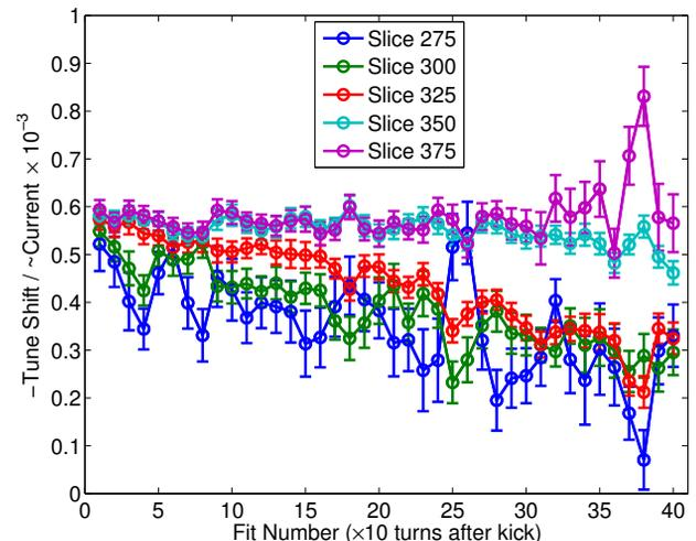
Figure 4: (Color) Normalized tune shift as a function of fit number for several slices along the bunch with one rms uncertainty. Slice 350 is the center of the bunch.
