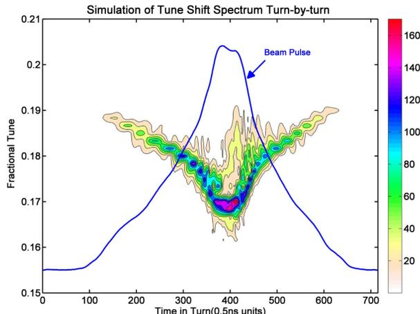
Figure 1: (Color) Simulation of tune distribution along the pulse using coherent space charge tune shift model Eq. (1) (contour) and measured longitudinal beam profile (blue line).
