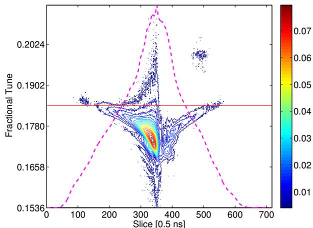
Figure 2: (Color) Measured tune distribution along the pulse (contour) and the last turn beam profile (dashed magenta line).
