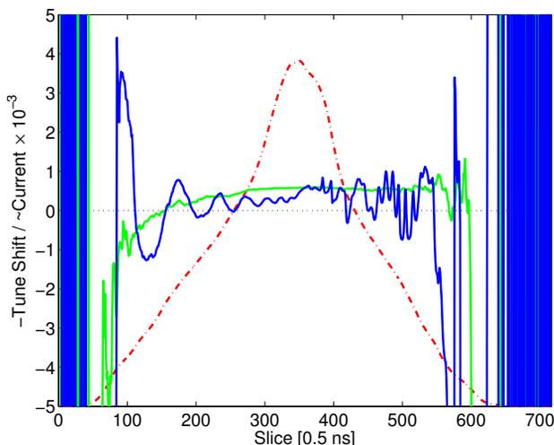
Figure 5: (Color) The measured normalized tune shift immediately after the single-turn kick (green) and 400 turns later (blue) as a function of slice along the bunch for bunched production-like beam with the RF buncher on and the last turn beam profile (red).
