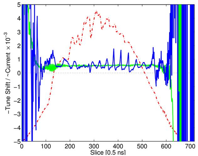
Figure 6: (Color) The measured normalized tune shift immediately after the single-turn kick (green) and 800 turns later (blue) as a function of slice along the bunch for bunched coasting beam with RF buncher off and the last turn beam profile (red).
