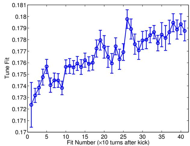
Figure 3: Fitted tune as a function of fit number (10 turn steps) after a single-turn kick for slice 300 ( $\sim 25$  ns in front of the peak) with one rms fitting uncertainty.
