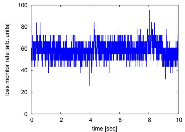
Figure 6: Loss monitor rates in the vicinity of the vertical collimator, sampled at 720 Hz.
