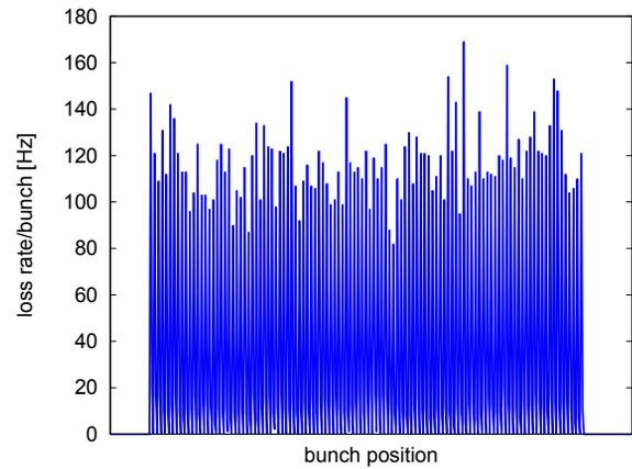
Figure 5: Bunch-by-bunch loss rates at a fixed point in time during the tune scan.
