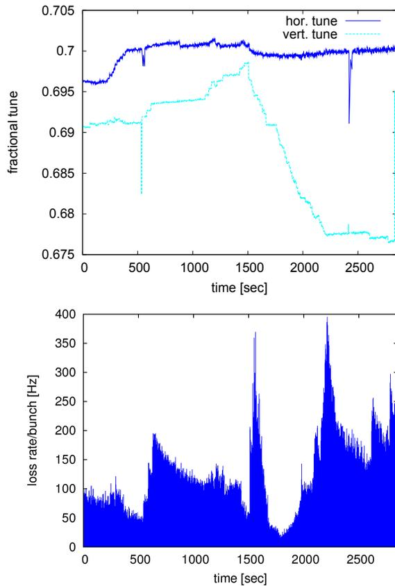
Figure 4: Loss rates during the tune scan. The horizontal scale is consistent with the one used in Figure 3, i.e. the tune scan starts after the collimators have reached their final position.
