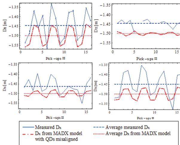
Figure 4: Comparison of the measured horizontal dispersion at the 16 pick-ups with the dispersions given by the PSB MADX model with misalignments of the QDs for ring 1 (top left), ring 2 (top right), ring 3 (bottom left) and ring 4 (bottom right).
