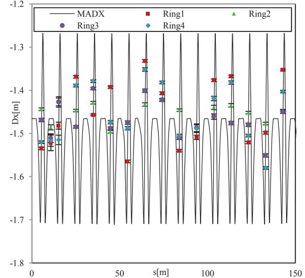
Figure 2: MADX simulation of the horizontal dispersion along the PSB ring (solid line) with the measurement points for the horizontal dispersion  $D_x$  for the 4 rings.
