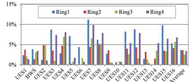
Figure 3: Relative differences of  $D_x$  given by the MADX model and obtained by measurements for the 4 rings. The pick-ups UES6 and UES10 of Ring2 are excluded from the analysis.
