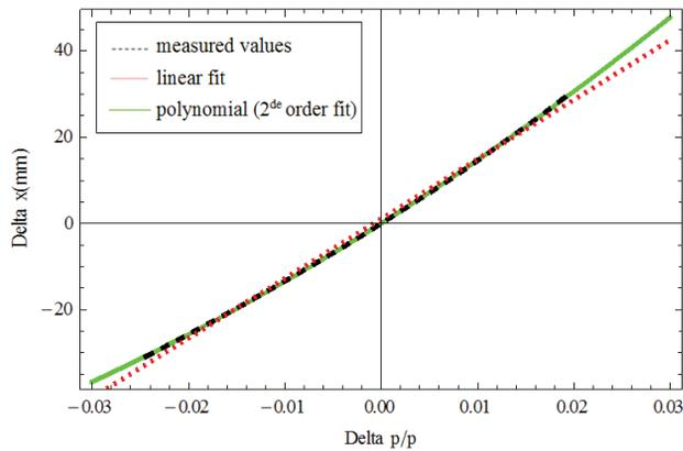
Figure 1: Plots of  $\Delta x$  vs.  $\delta$  resulting from measurements done on the pick-up BR1.UES5L3 using the simplified relation  $\Delta f/f_0 = -\eta_0 \cdot \delta$ .
