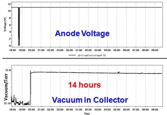
Figure 5: 80 kHz modulator test with more than a 1A beam.
