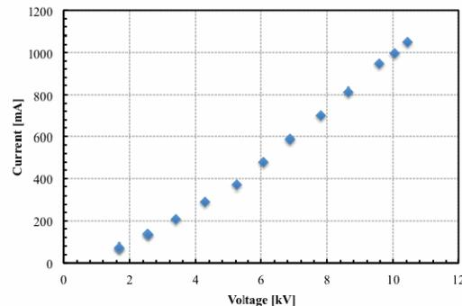
Figure 4: Perveance measurement of the electron gun.
