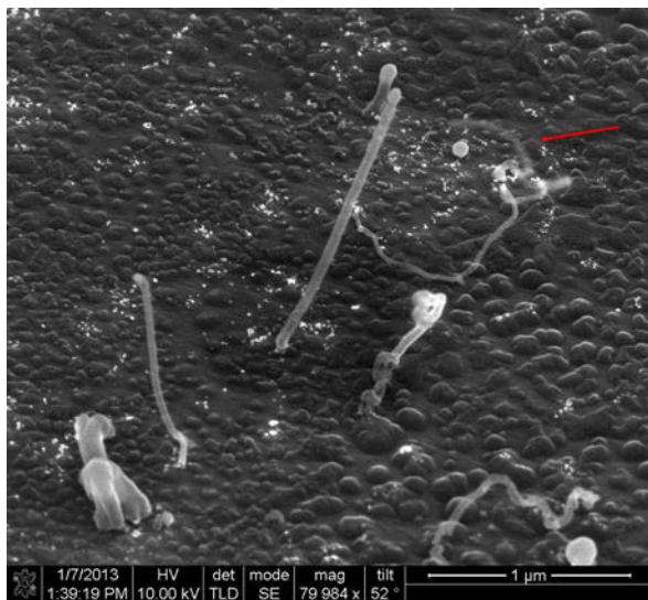
Figure 3: CNTs deposited onto a copper substrate via CVD. The red arrow points to a blurred CNT, indicating that it was only attached at one end, and was free to vibrate in the SEM.
