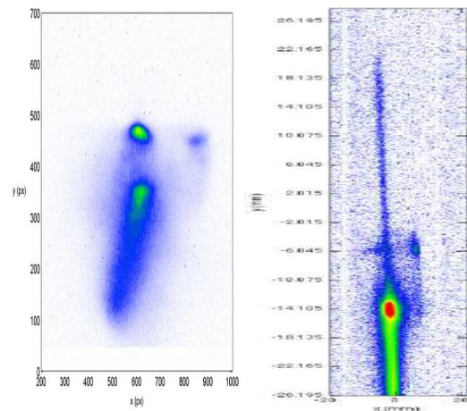
Figure 4: Left: Accelerated witness beam (top feature) with decelerated drive beam (bottom feature) produced in a pre-formed lithium plasma. Right: Energy doubled tail with decelerated beam core produced in self-ionized plasma generated in argon gas. In both plots energy increases with height.
