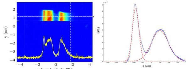
Figure 2: Spectral profile of the electron beam (left) and longitudinal profile of the electron beam (right) after notch collimation and before entering the plasma source.
