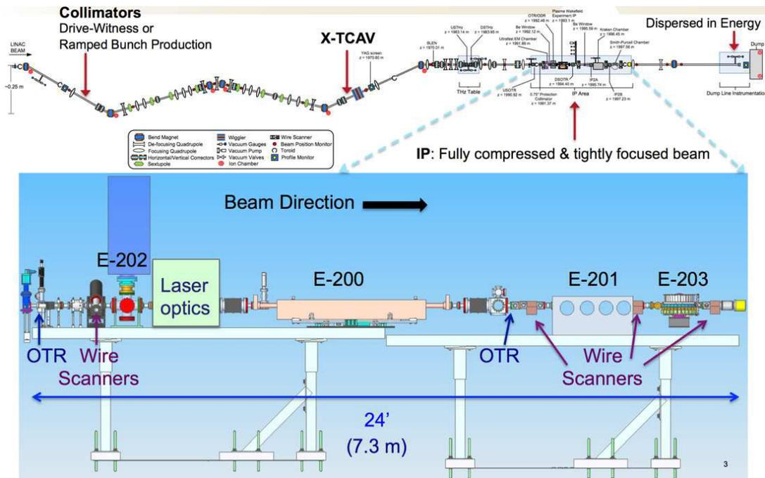
Figure 1: Top: The FACET beamline. Bottom: Detail of experimental area. The text “E200” marks the location of the plasma source.
