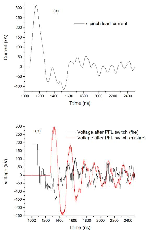
Figure 3: LTspice simulations of an ISIS-based x-pinch driver: (a) current measured at the x-pinch load (b) voltage measured after PFL switch.
