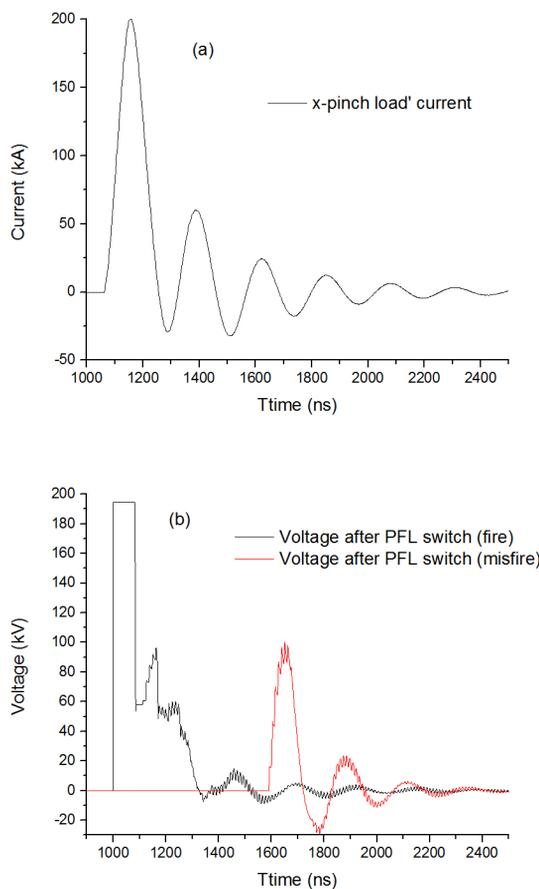
Figure 4: LTspice simulations of the ISIS-based  $x$ -pinch driver with a damping resistor placed after each PFL: (a) current measured on the  $x$ -pinch load (b) voltage measured after PFL switch.
