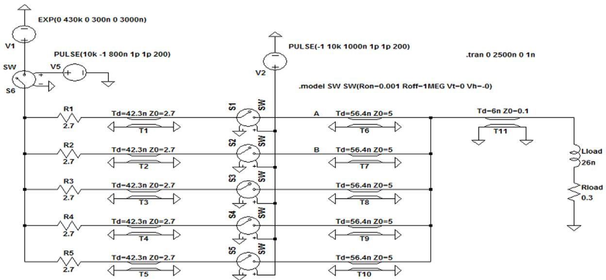
Figure 2: Electrical circuit of an ISIS-based x-pinch driver.
