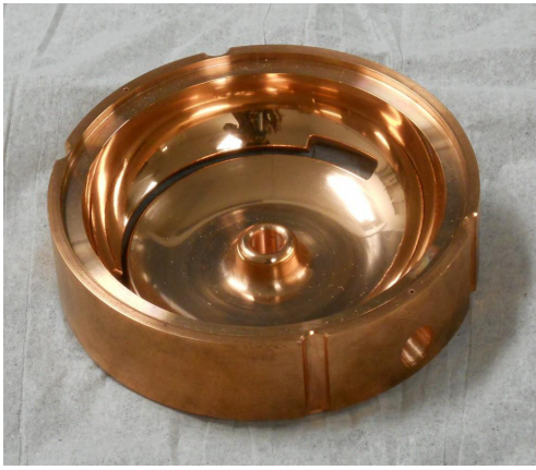
Figure 3: A finished half-cavity copper part.
