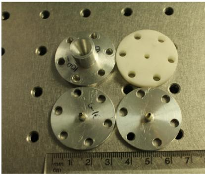
Figure 3: Nozzles used (diameters given). From left: (top) 10 mm conical nozzle, insulator (bottom) 2.5 mm by 1 mm slit nozzle, 2 mm conical nozzle.
