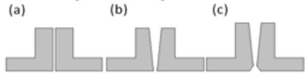
Figure 9: Supersonic slits: These are formed from two pieces as opposed to the single piece structure of the originals allowing the entrance aperture and nozzle diameter to be varied. Shown are the prism faces of each and all have a depth of 35 mm: (a) 15 mm x 15 mm (b) 15 mm x 15 mm with wall angle of 2° (c) 18 mm x 15 mm with wall angle 2° and lower of 65°.
