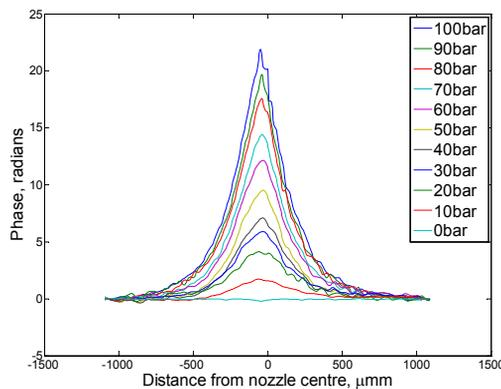
Figure 8: Phase line out 1 mm above nozzle normal to laser and gas jet for 2.5 mm x 1 mm slit nozzle at normal incidence.
