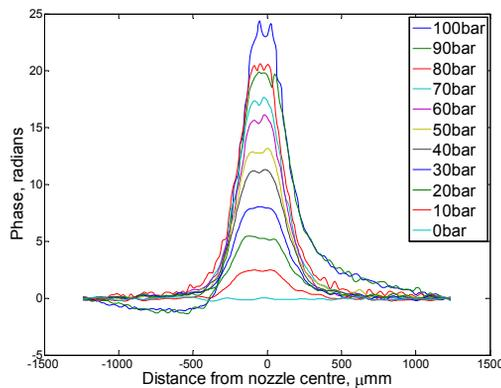
Figure 7: Phase line out 1 mm above nozzle normal to laser and gas jet for 2.5 mm x 1 mm slit nozzle at normal incidence.
