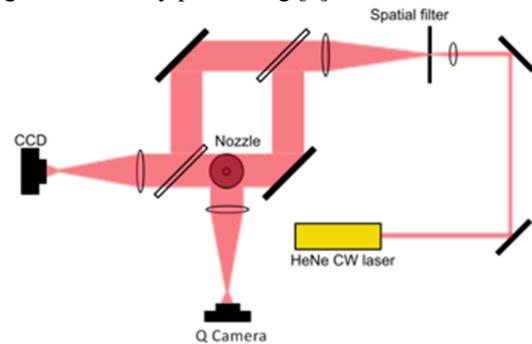
Figure 4: Experimental set up used. Combining Mach-Zehnder interferometry with an additional focussing lens and camera to image Rayleigh Scattering from the probing laser due to clusters within the gas medium.
