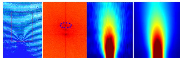
Figure 5: Interferometry image processing (from left): 1 showing region selected for transforming (red box), 2 showing Fourier transformed phase map with sample area highlighted (blue ring), 3 gas jet density profile, 4 smoothed density profile with geometric compensations.
