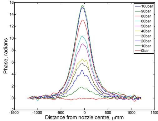
Figure 6: Phase line out 1 mm above nozzle normal to laser and gas jet for 2 mm diameter sonic nozzle.
