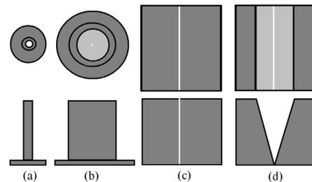
Figure 2: Examples of nozzle geometries for (a) sonic nozzle (b) conical nozzle (c) slit nozzle (d) supersonic slit nozzle.
