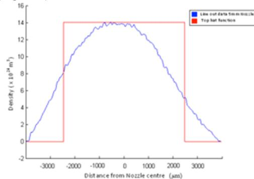
Figure 1: Ideal gas jet would possess a density profile that follows the shape of a top hat function. Actual jets do not produce such a steep density gradient.
