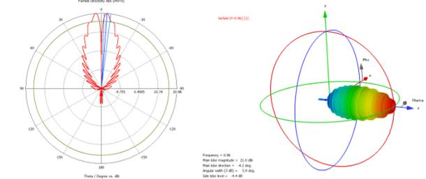
Figure 5: Circular pattern and 3D diagram for maximal directivity of circular antenna.
