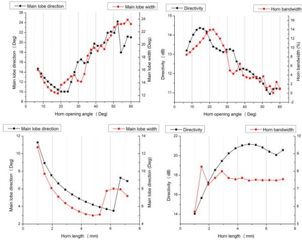
Figure 3: Dependences of electrodynamic characteristics vs. circular horn geometrical sizes.
