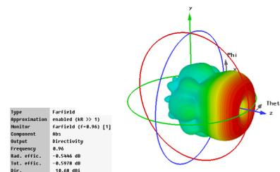
Figure 1: Directivity diagram of the open capillary end.
