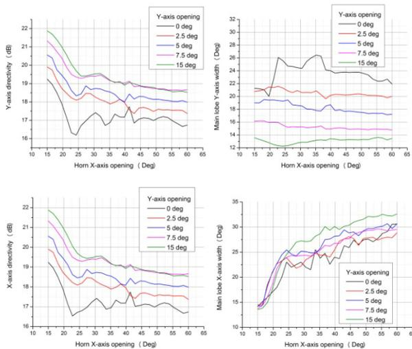
Figure 8: Dependences of electrodynamics characteristics vs. rectangular horn geometrical sizes.
