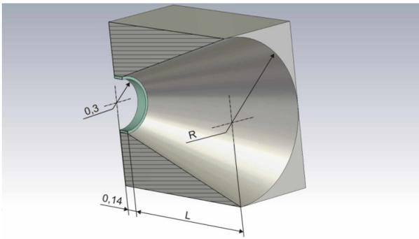
Figure 2: Circular horn antenna and the capillary.
