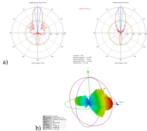
Figure 10: Circular pattern in horizontal plane (a - left), in vertical plane (a - right) and 3D directivity diagram for maximal main lobe angular width of rectangular antenna.
