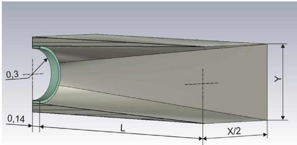
Figure 7: Horn antenna with circular to rectangular cross section transition and the capillary.
