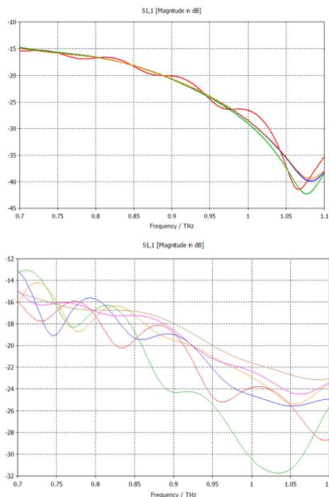
Figure 4: Reflection coefficients of the horn for different geometrical sizes of the horn.
