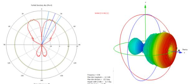
Figure 6: Circular pattern and 3D diagram for maximal main lobe angular width of circular antenna.
