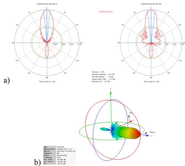
Figure 9: Circular pattern in horizontal plane (a - left), in vertical plane (a - right) and 3D directivity diagram for maximal directivity of rectangular antenna.
