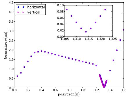
Figure 3: Beam size as a function of distance from cathode.
