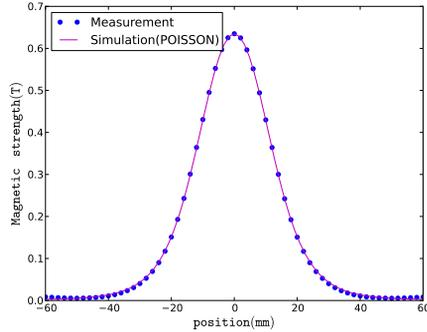
Figure 2: Magnetic field of Solenoid 2.
