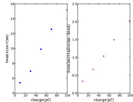
Figure 5: Beam size (left) and normalized emittance (right) as a function of beam charge.
