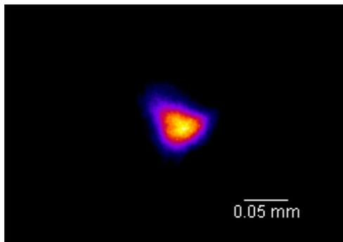
Figure 7: Beam profile measured by HD-810 film.
