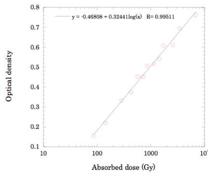
Figure 6: Calibration curve of HD-810 film.
