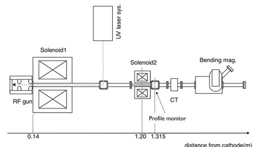
Figure 1: Schematic design of Waseda beam line.
