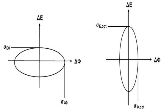
Figure 1: Phase space before & after compression.
