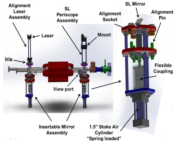
Figure 5: Chamber with laser & SL assembly.
