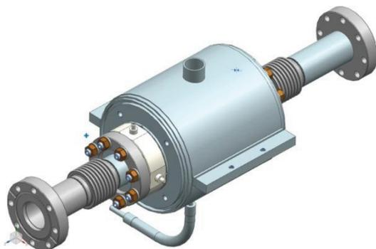
Figure 6: Focusing solenoid and BPM.
