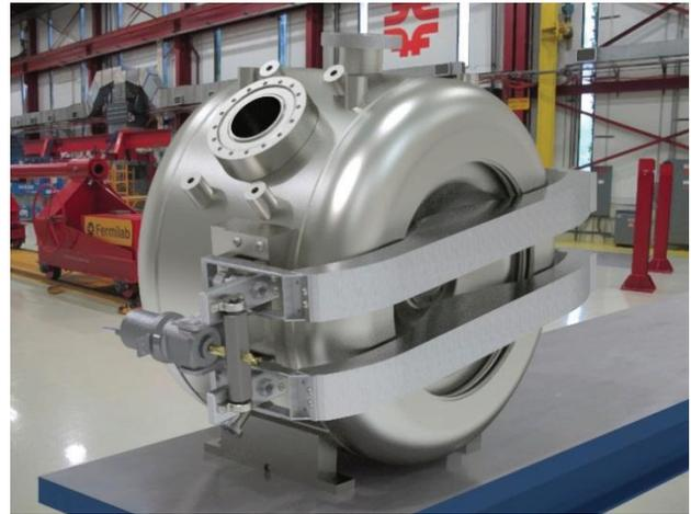
Figure 3: Dressed cavity and tuner.
