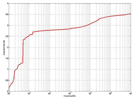
Figure 2: Integrated added jitter.
