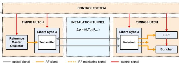
Figure 4: Example of use an accelerator environment.
