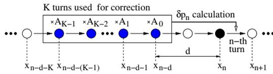
Figure 2: Schematic diagram representing the work of digital filter. Correction algorithm uses  $\mathcal{K}$  turns of prehistory (blue circles) in order to calculate the change in momentum  $\delta p_n$ , which will be applied  $d$  turns later (for this diagram  $d = 2$ ) after the current turn ( $n$ -th turn shown with a black filled circle).
