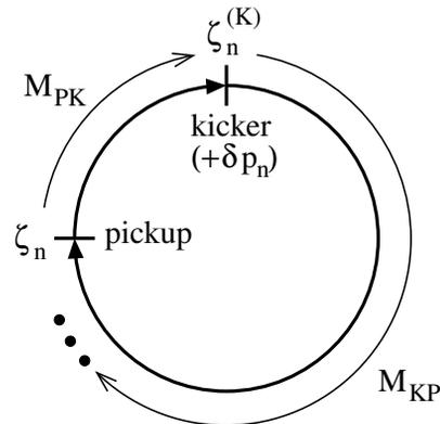
Figure 1: Schematic plot of the one turn transformation of the betatron state-vector in a lattice with damper.
