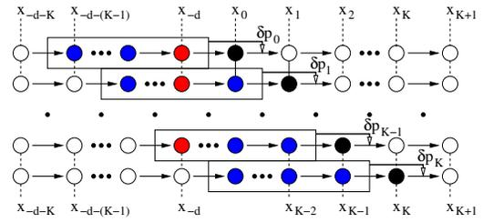
Figure 3: Schematic diagram representing the work of digital filter for  $\mathcal{K}$  turns with single erroneous measurement ( $(-d)$ -th turn shown with a red circle).
