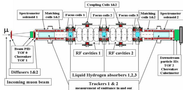
Figure 1: Layout of the MICE cooling cell. It is a prototype of a cooling channel section for use in a Neutrino Factory or a Muon Collider.
