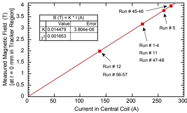
Figure 6: Magnetic field linearity study.
