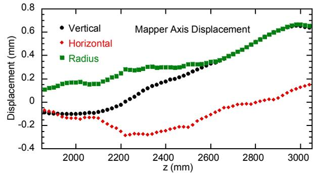
Figure 8: Survey of magnet measurement device axis (zoom-in on tracker region) in a coordinate system aligned to the cold mass axis.
