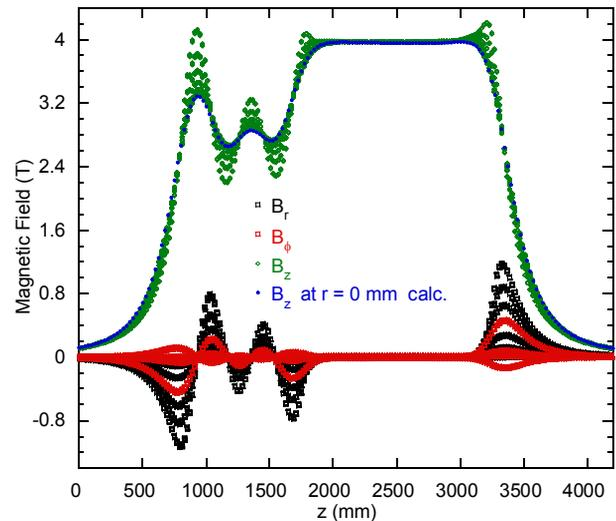
Figure 5: Measured field components for all probes, and a numerical calculation of the longitudinal field on magnetic axis using "as-built" coil parameters.
