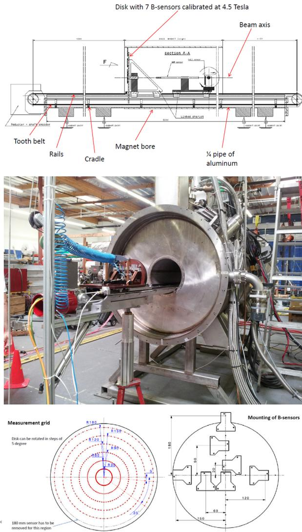
Figure 4: (Top) Magnet measurement device setup. (Center) Photo of the system in use for SS2 magnet. (Bottom left) Measurement grid of the device. (Bottom right) Mounting positions of the seven 3D Hall probe sensors on the disk.
