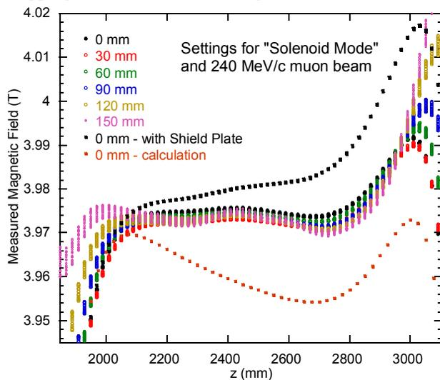
Figure 7: Longitudinal magnetic field component in the tracker region: measurements for 3D Hall probes at different radii for a case without shielding plate, measurements at 0 mm for a case with shielding plate, and a numerical calculation on axis (no shielding plate) using “as-built” coil parameters and measured coil currents.
