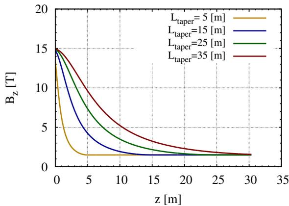
Figure 3: On-axis magnetic field profiles for the Target System.
