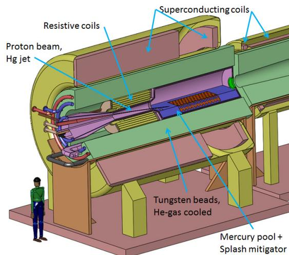
Figure 2: Neutrino Factory/Muon Collider target system.
