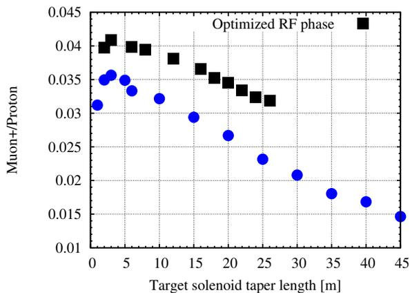
Figure 6: Muon yield from the Front End, within the acceptance of the accelerator chain vs. the solenoid taper length. The RF optimization (black curve) increased the Front End performance by  $\approx 16\text{-}40\%$ .
