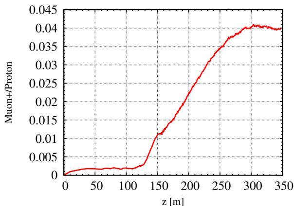
Figure 5: Number of muons within the accelerator-chain acceptance at various distances along the Front End.
