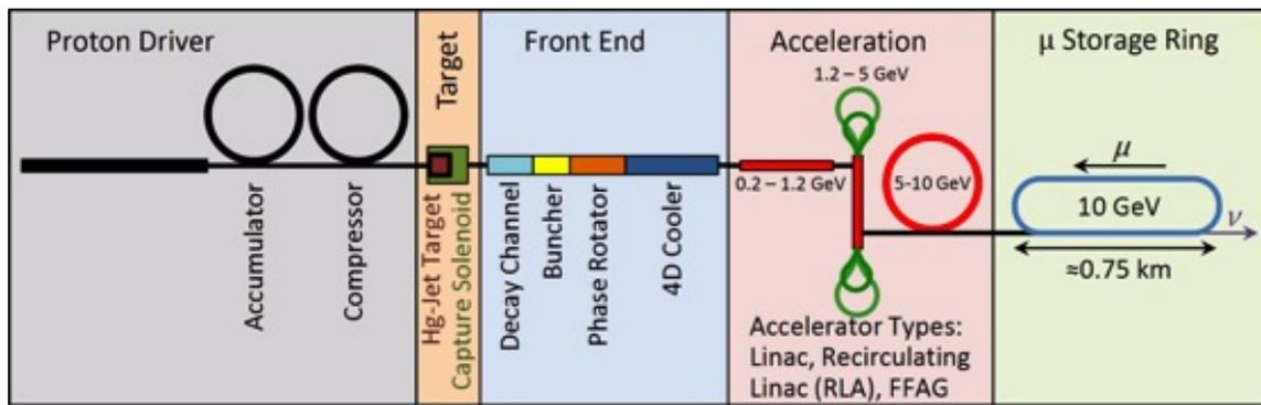
Figure 1: Neutrino Factory/Muon Collider Target System.
