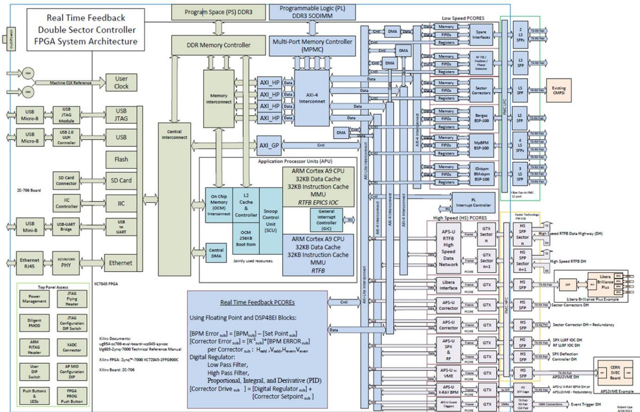
Figure 3: RTFB DSC FPGA architecture using Zynq-XC7Z045 FPGA.
