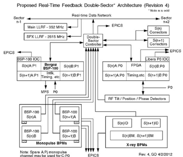
Figure 1: Real-time feedback double-sector controller architecture.
