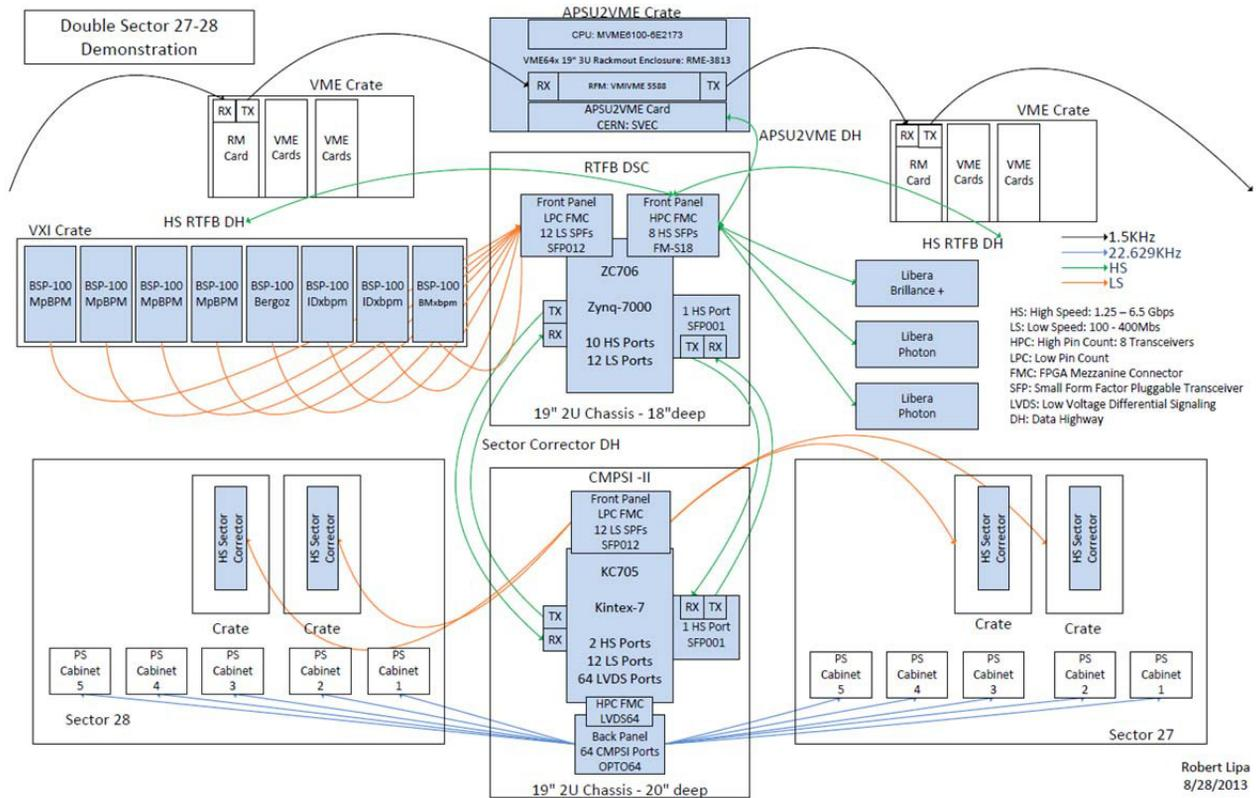
Figure 2: RTFB system architecture implementation using three chassis.
