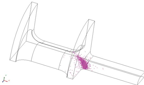
Figure 5: Particle distribution after 30 RF cycles in the multipacting band, showing accumulation of resonant particles near the fillet between cavity and beampipe.
