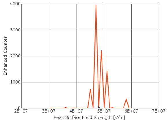
Figure 6: Enhanced counter function (number of particles surviving to 20 impacts including yield) as a function of peak surface electric field.
