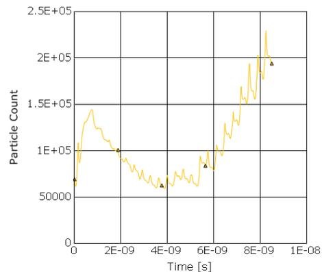
Figure 7: Particle count vs. time in deflector at 49 MV/m. Resonance is evident in late-time growth.
