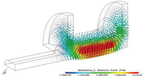
Figure 4: Electric field of mode in deflector cavity. Cavity is shown as modelled using 3 planes of symmetry. View is combination of structure and field annotations.
