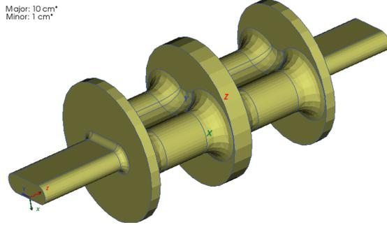
Figure 3: Deflector cavity geometry.
