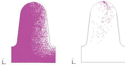
Figure 1: Particle cloud at 1 RF period (left), and after 2 RF periods (right) in 2-D RZ example. Ultimately a resonance is seen about cavity “equator” (top center of cavity).
