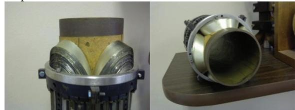
Figure 3: Photograph of coil ends of a test quadrupole magnet wound with Nb<sub>3</sub>Sn tape.
