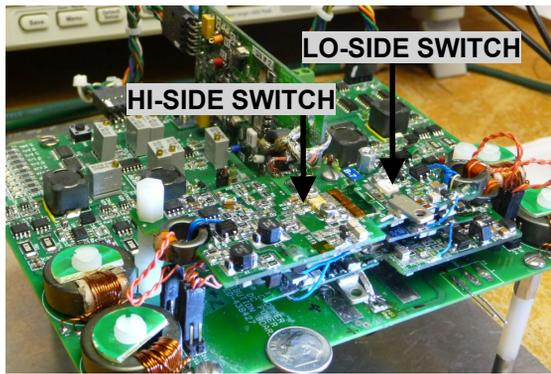
Figure 3: Bipolar switch composed of 3-FET cascode switches mounted to power distribution board.
