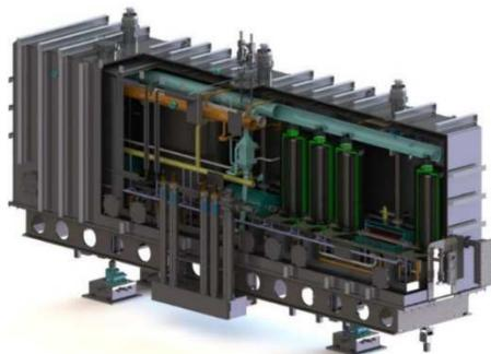
Figure 1: Cross-Section of ReA6  $\beta=0.085$  QWR Cryomodule.
