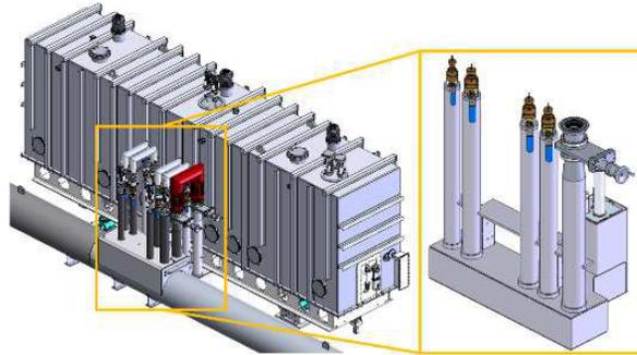
Figure 2: Cryomodule bayonet box interface to the helium distribution line.
