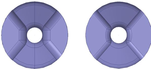
Figure 5: The cross section of the original RF dipole geometry, with flat inner ridges on the left and the modified separator cavity shape on the right, showing the curved faces of the inner ridge.
