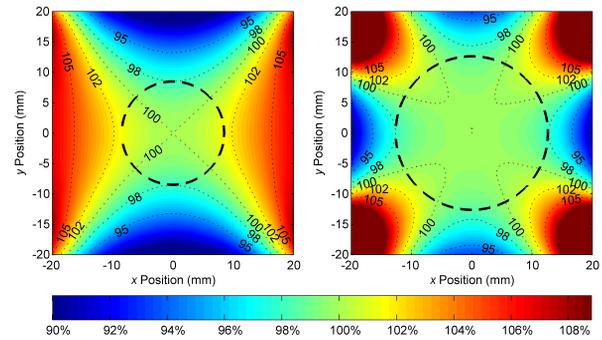
Figure 6: A comparison of the kick-uniformity for the RF dipole with flat ridge geometry on the left, and curved ridges on the right. The dashed circle shows the area in which the momentum kick is within 2% of the on axis kick strength.
