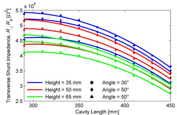
Figure 4: The transverse shunt impedance for varying ridge height and angle and the cavity length.
