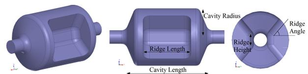
Figure 1: The RF dipole geometry showing the key parameters affecting the cavity performance.
