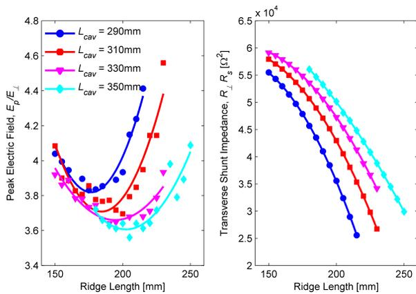
Figure 2: The peak electric fields on the left, and the transverse shunt impedance on the right for varying ridge and cavity lengths. For reference:  $\beta\lambda/2 = 230$  mm at 650 MHz.
