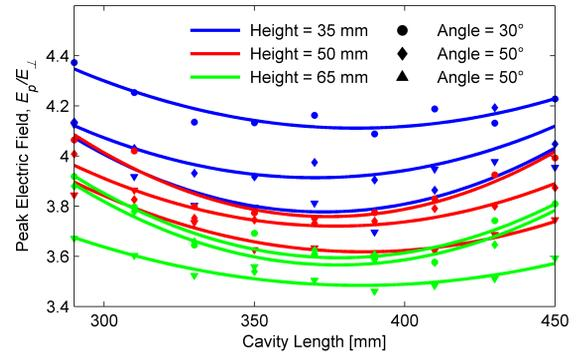
Figure 3: The peak electric fields for varying ridge height and angle and the cavity length. The colour of the line indicates the ridge height and the shape of the data point the angle of the ridge.
