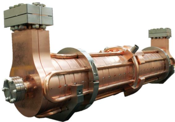
Figure 4: Picture of the PAL deflector after the final brazing and before installation.
