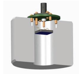
Figure 2: LANL PIN diode assembly.
