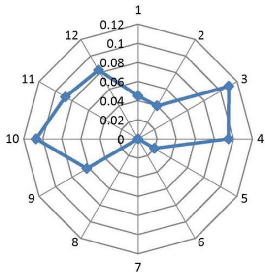
Figure 7: Circular plot of peak PIN diode signals during an abnormal injector event.
