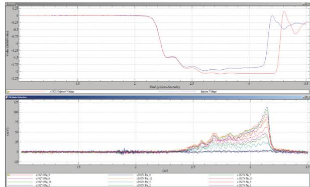
Figure 6: Injector voltage waveforms. Top waveform showing normal (red) and droop (blue) conditions. Bottom waveform shows PIN diode signals recorded during injector voltage droop.
