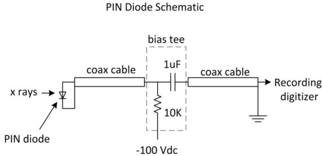
Figure 5: PIN diode schematic.
