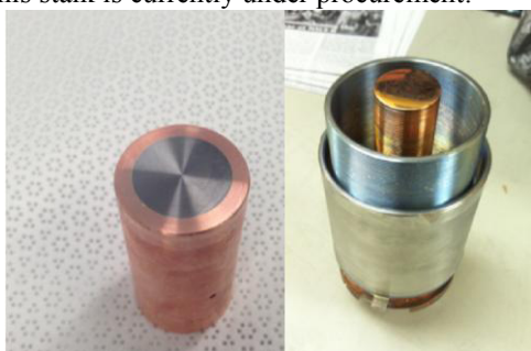
Figure 3: Left – the dummy brazed Ta-Cu sample; Right – the polished copper cathode stalk with the choke joint section.
